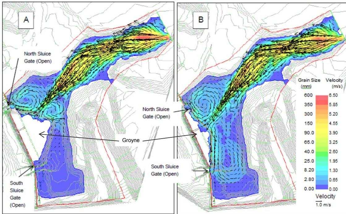
Figure 3. Sediment deflection groyne – flow paths and velocities through both the north and south sluice gates: A) 30 m long groyne and B) 15 m long groyne.
