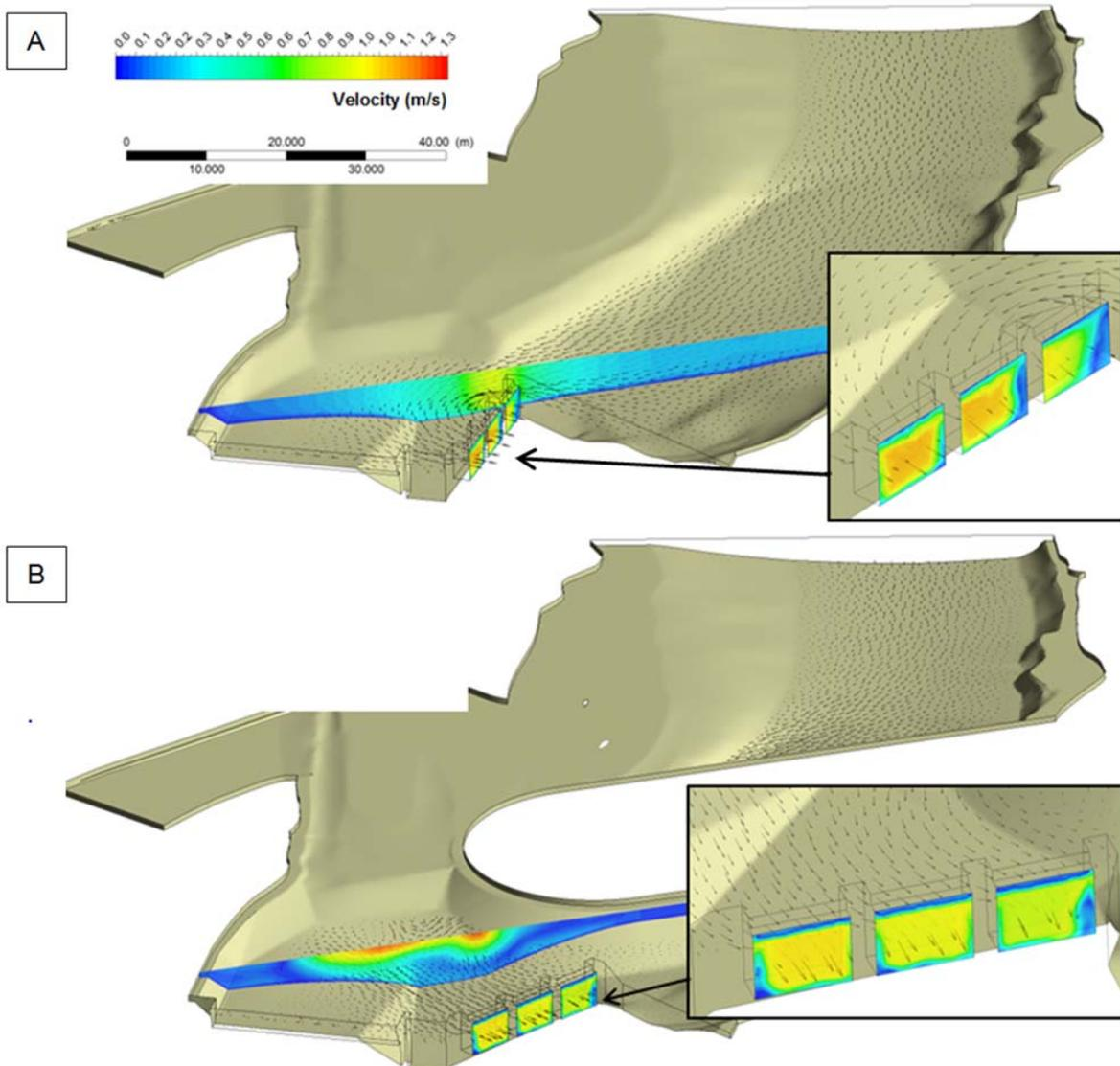
Figure 8: Velocity distribution for Intake B: (A) without a sediment deflection berm, and (B) with a sediment deflection berm
