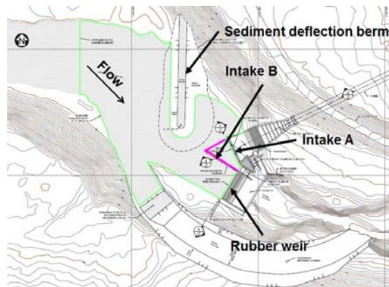
Figure 6: CFD model setup with the key intake elements
