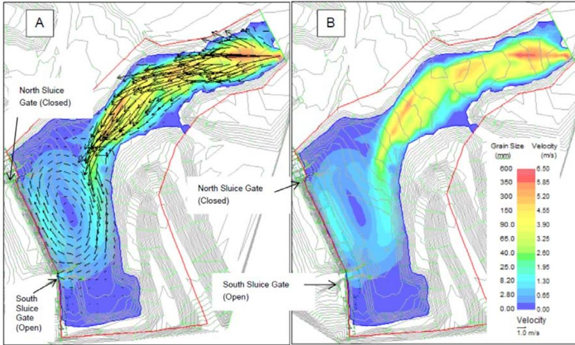
Figure 2. Additional sluice gate – flow only through the south sluice gate: A) Flow paths and velocities; and B) Mobile sediment grain sizes.
