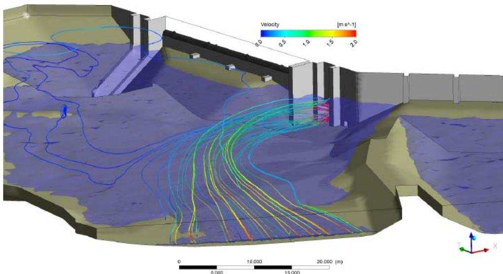
Figure 4: Streamlines through the headpond for sluicing activities
