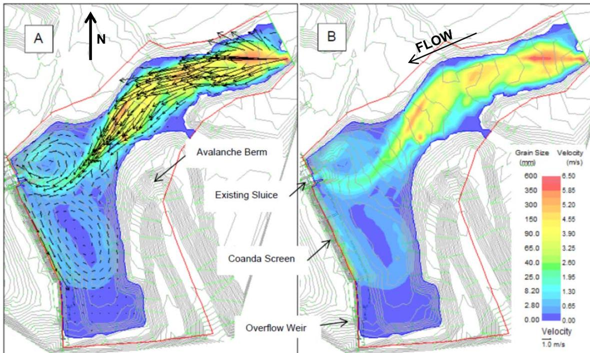
Figure 1. Baseline model – flow through the existing north sluice gate: A) Flow paths and velocities; and B) Mobile sediment grain sizes.
