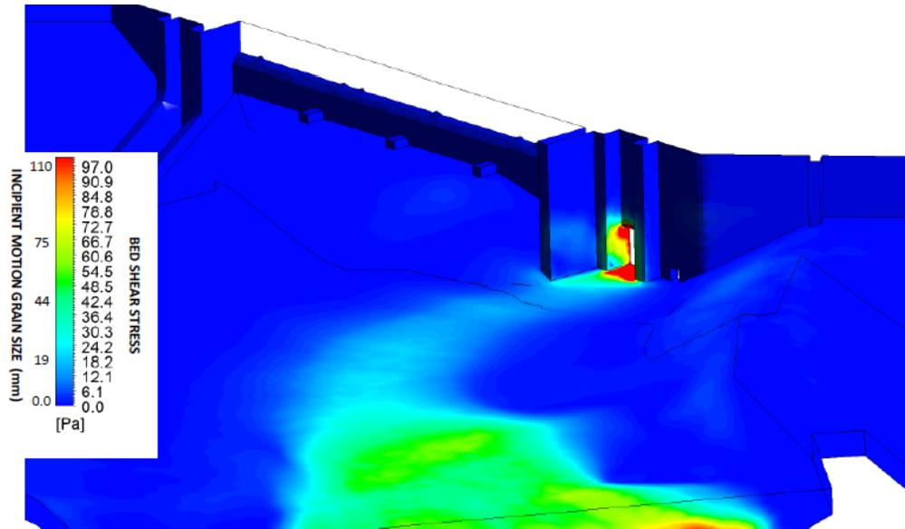
Figure 5: Shear stresses through the headpond for sluicing activities
