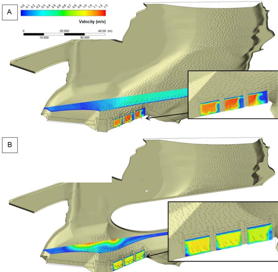
Figure 7: Velocity distribution for Intake A: (A) without a sediment deflection berm, and (B) with a sediment deflection berm
