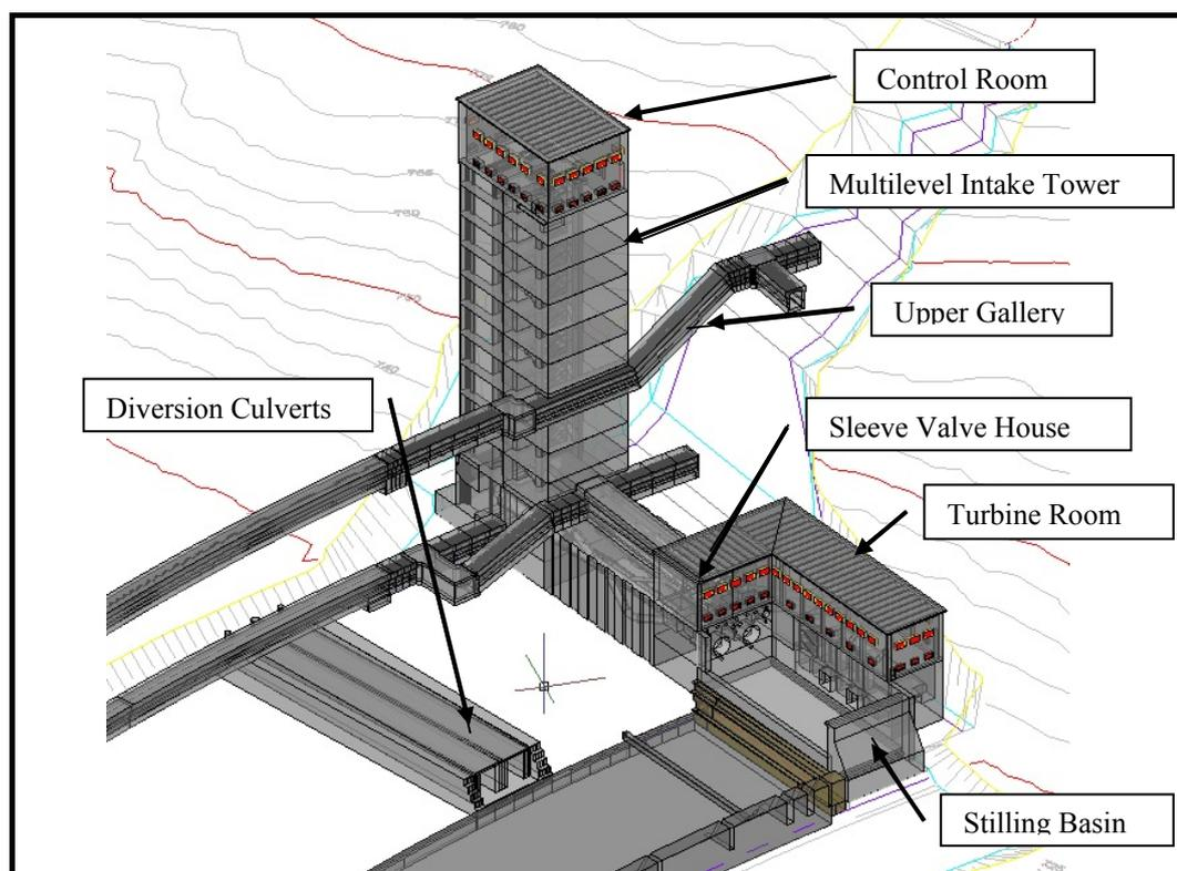
*Figure 5.1: Neckartal Dam Outlet Works (isometric view)*
