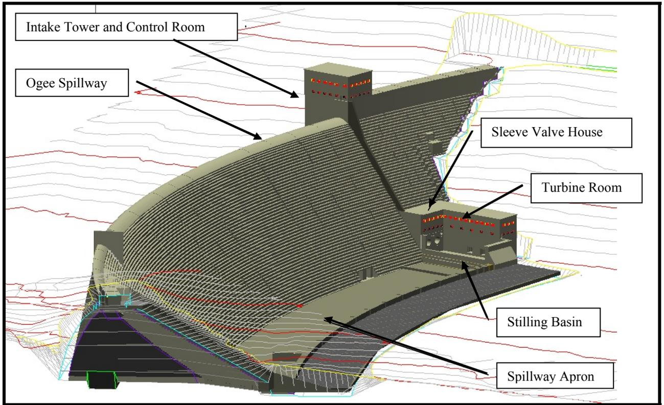
*Figure 1.1: Neckartal Dam (Isometric view)*
