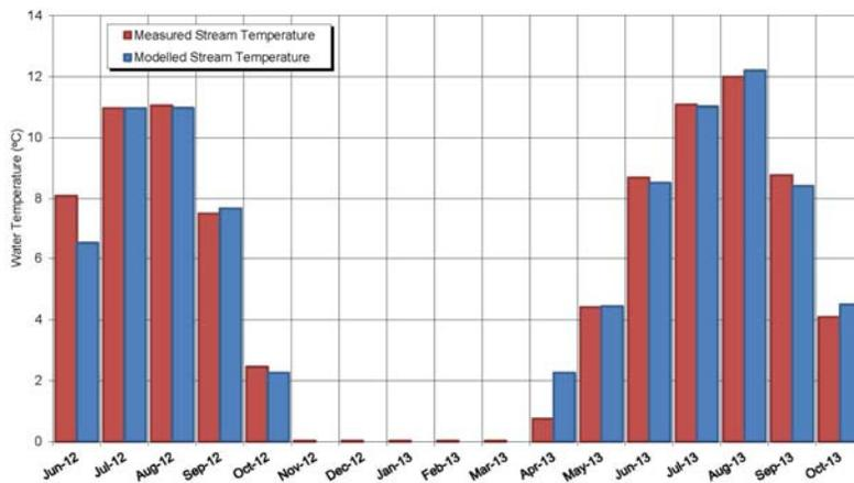
Figure 3: Temperature calibration of the Creek model.
