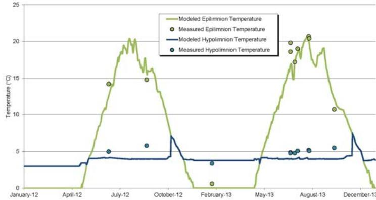
Figure 2: Temperature calibration of the Lake model.
