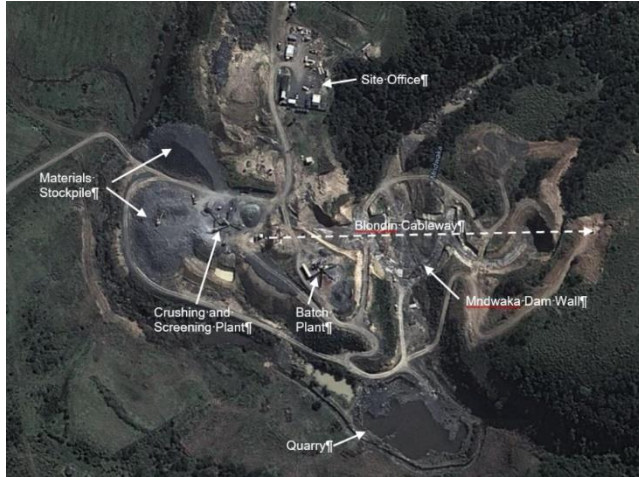
Figure 6. Mndwaka Dam – site layout
