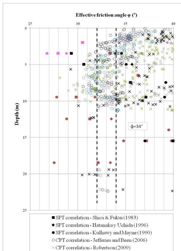
Figure 9. Effective friction angle for coarse material
