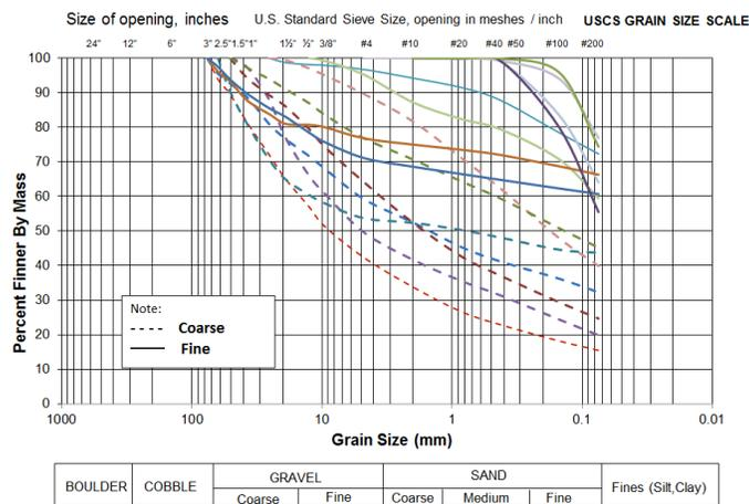
Figure 5. Grain size distribution of representative samples
