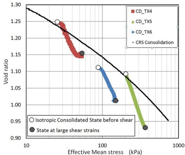
Figure 6. Compilation of the state curves for triaxial tests on Fine tailings, along with the consolidation relationship observed in CRS consolidation on the material.
