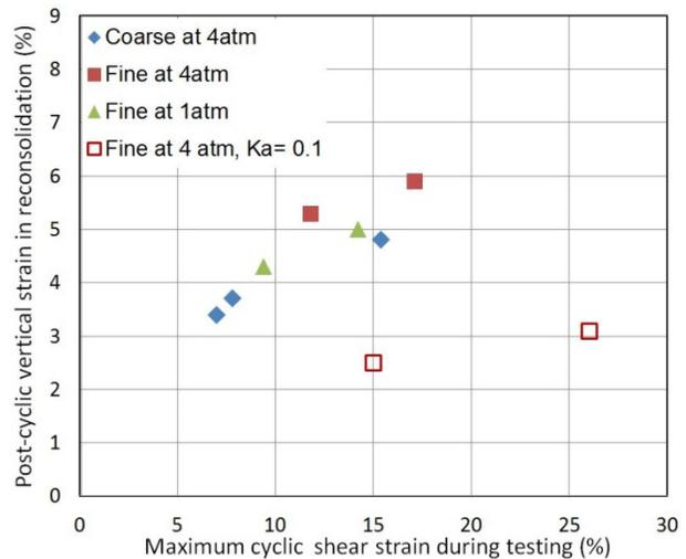
Figure 5. Reconsolidation strains after CSS testing.
