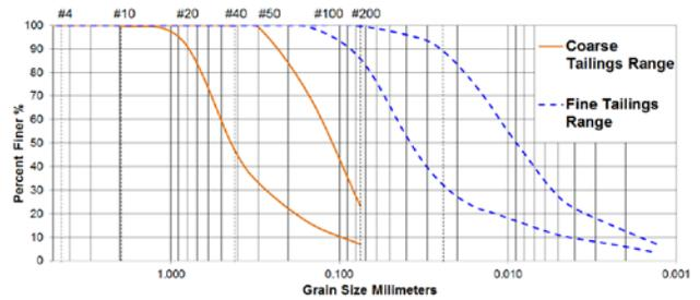
Figure 2. Grain Size ranges of Tailings
