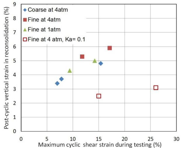
Figure 5. Reconsolidation strains after CSS testing.
