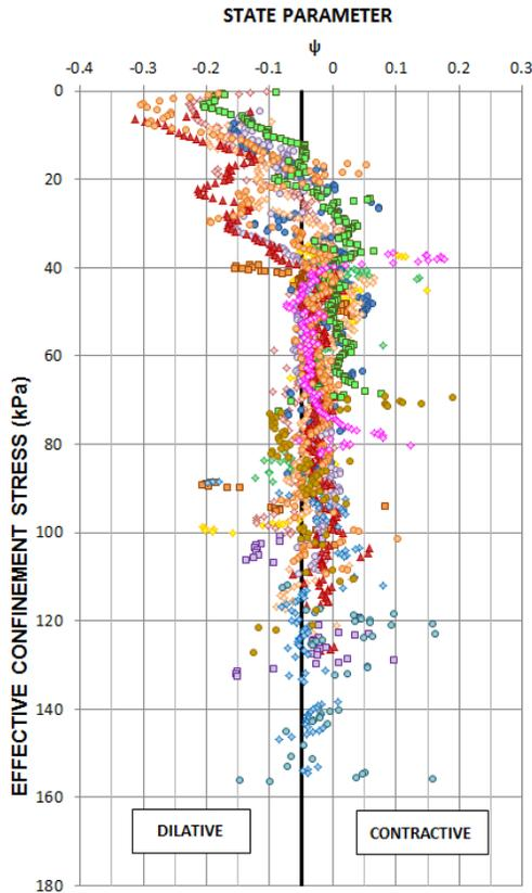
Figure 1. Estimated state parameter based on CPTU correlation
