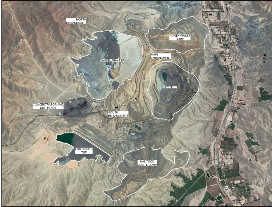
Figure 1. General Mine Site Arrangement
