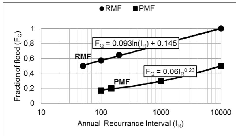
Figure 3. The functions representing the fractions of the RMF and PMF against annual recurrence interval (I<sub>R</sub>). Functions representing the RMF and PMF fraction-curves are indicated by F<sub>Q</sub>
