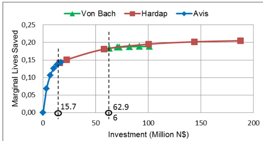
Figure 7. The combined ITC's for the Hardap, Von Bach and Avis Dams. Indicated are the transition points for investment from one dam to the next to optimise expenditure
