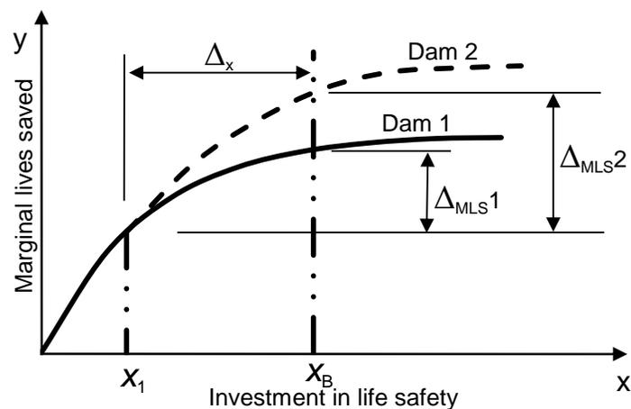
Figure 3. Optimising risk reduction by applying the RQO process. Where  $X = XD2$ , investment in rehabilitation is shifted from Dam 1 to Dam 2. Therefore at  $X_B$ , the budget limit, more marginal lives have been saved through the optimising process than having the investment remain with Dam 1
