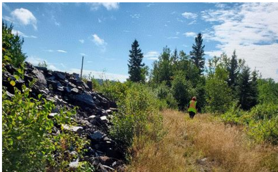
Photo 6. Waste rock sampling for ARD and ML testing
