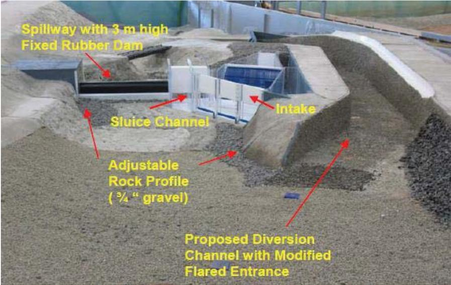
**Figure 4. Physical Model Constructed and Tested for the 33 MW Upper Stave River HEF**
