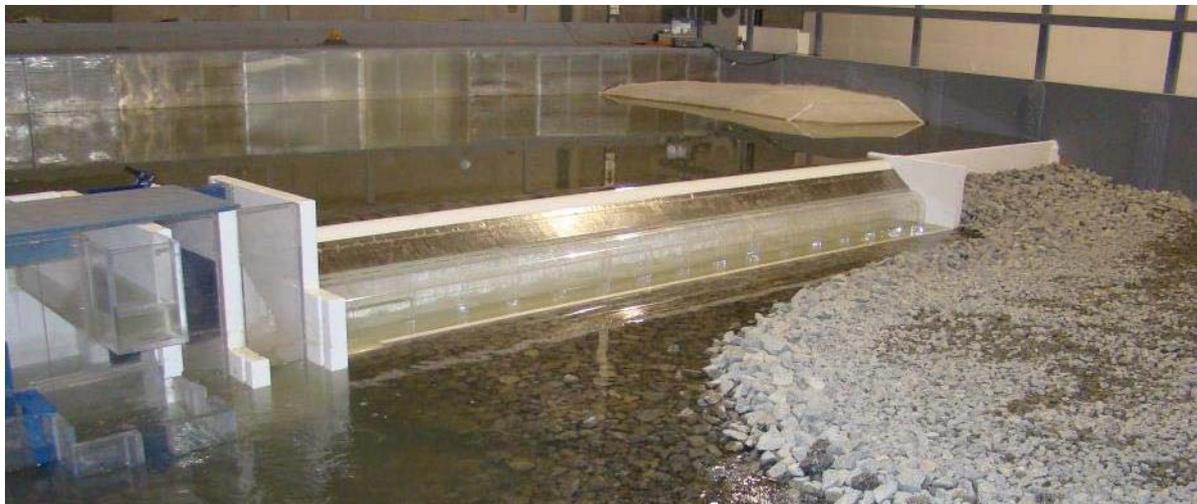
**Figure 8. Kokish River Intake Physical Model**
