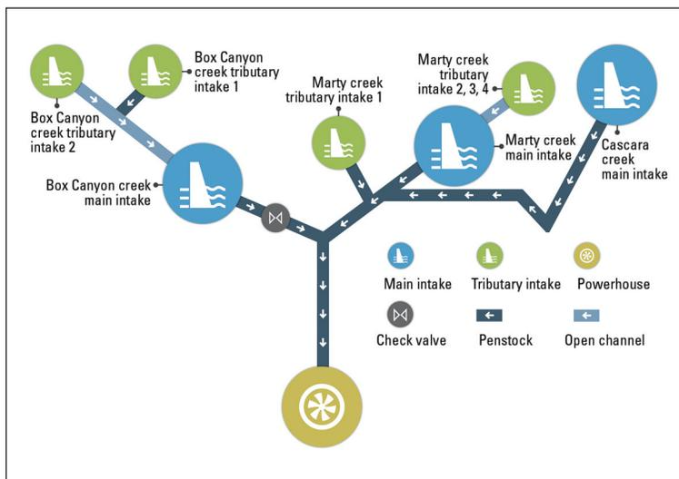
Fig. 2. Schematic highlighting the complexity of the Box Canyon project.
