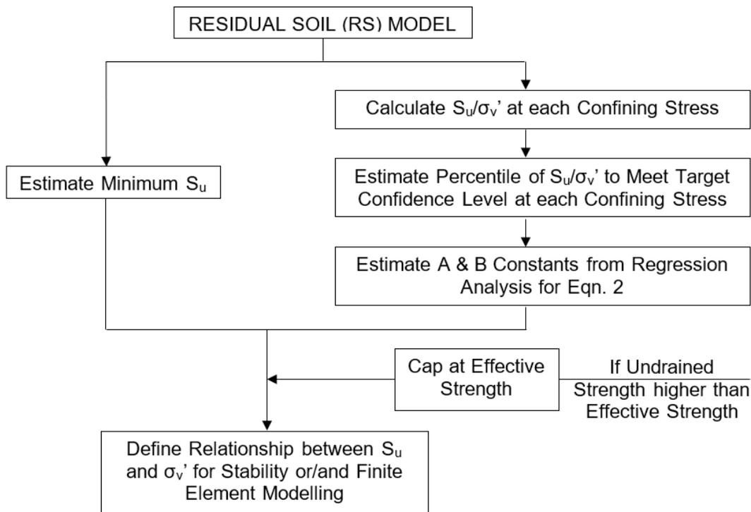
FIG 2 – Methodology to Estimate Residual Soil (RS) Model Parameters
