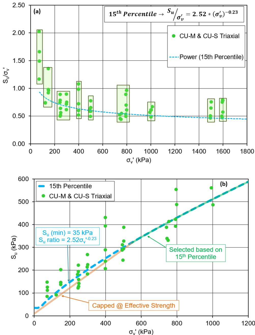
FIG 3 – Parameter Estimation: (a) A & B regressions and (b) Relationship between  $S_u$  &  $\sigma_v'$
