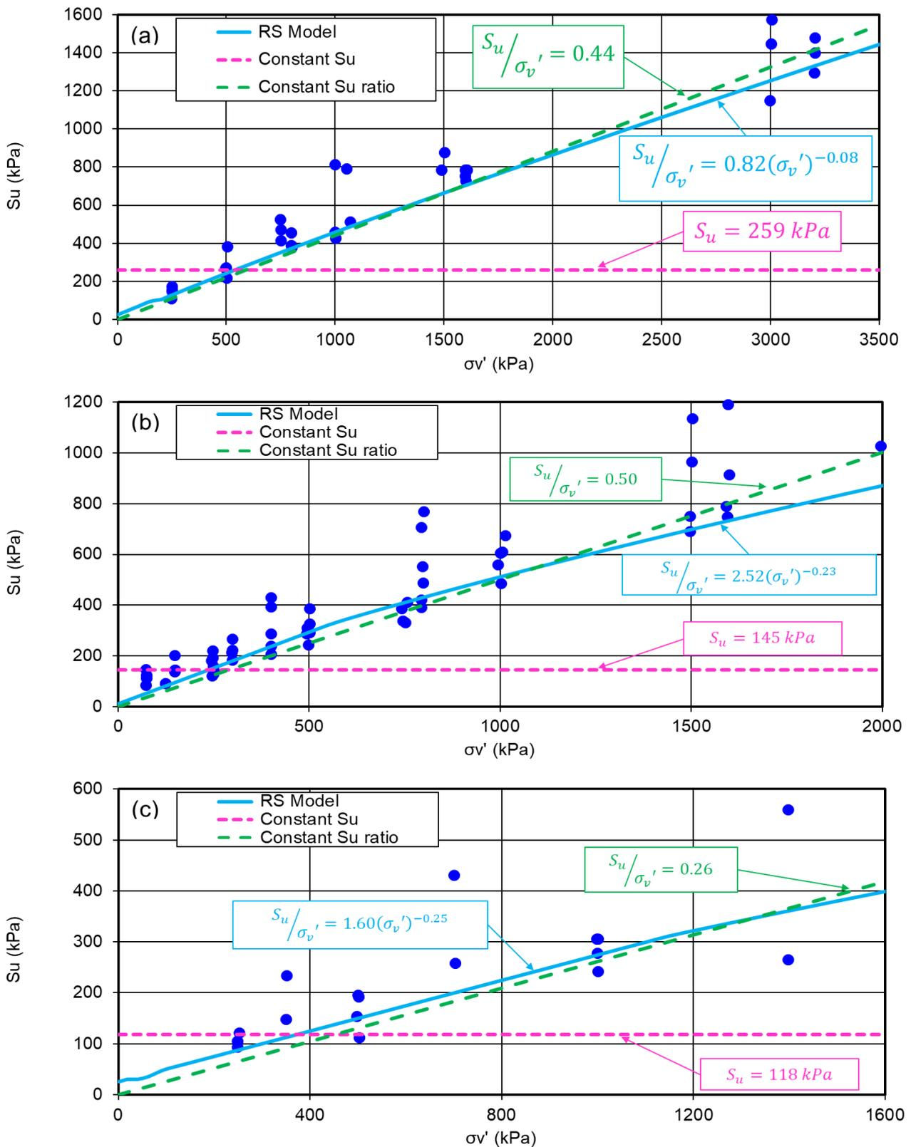
FIG 4 – Constant  $S_u/\sigma_v'$ , Constant  $S_u$  and RS Model (a) Siltstone (b) Greywacke (c) Monzonite
