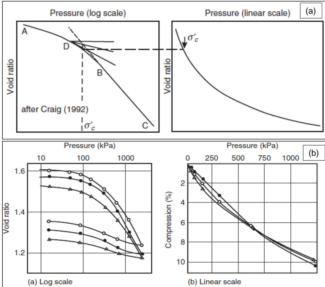
FIG 1 – Typical Oedometer Data Interpretation: (a) Sedimentary Soils and (b) Residual Red Clays (After Wesley, 2010)
