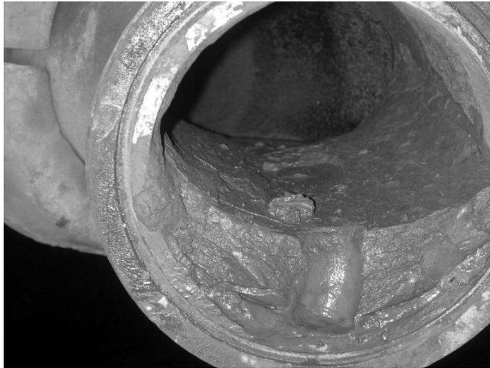
**Figure 4** Laminar flow settling in paste fill pipeline
