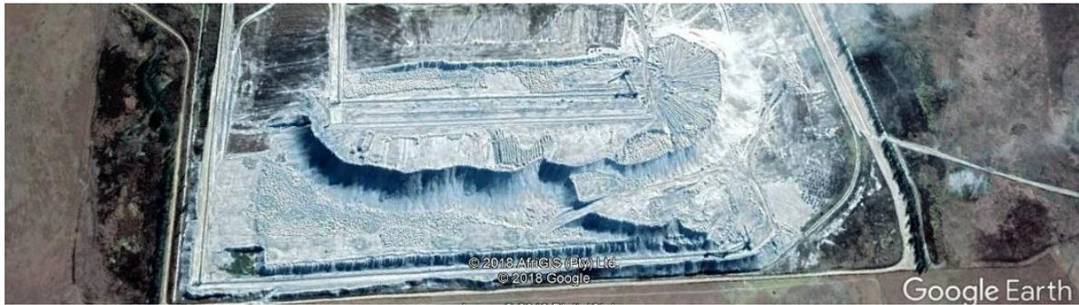
Figure 10 Google Image of ash dump with twin face conveyor system to form multiple lifts
