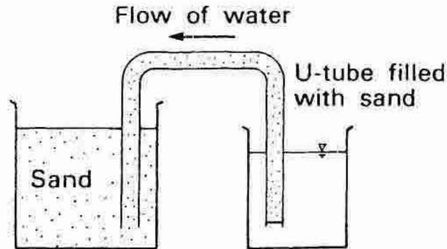
**Figure 1.23** Beaker and sand-filled glass tube for demonstrating the phenomenon of capillary flow through a sand (from Hogen-togler and Barber).
