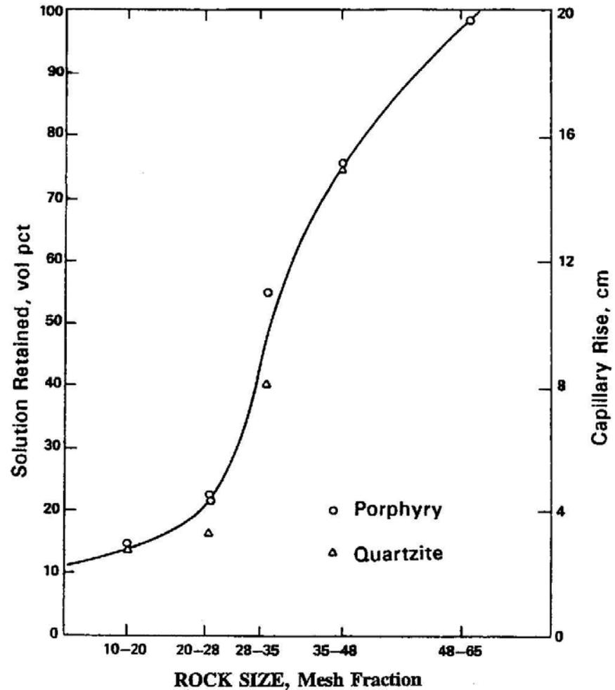
Figure 7.2. Solution retention and capillary rise as a function of rock fragment size (Schlitt, 1984).
