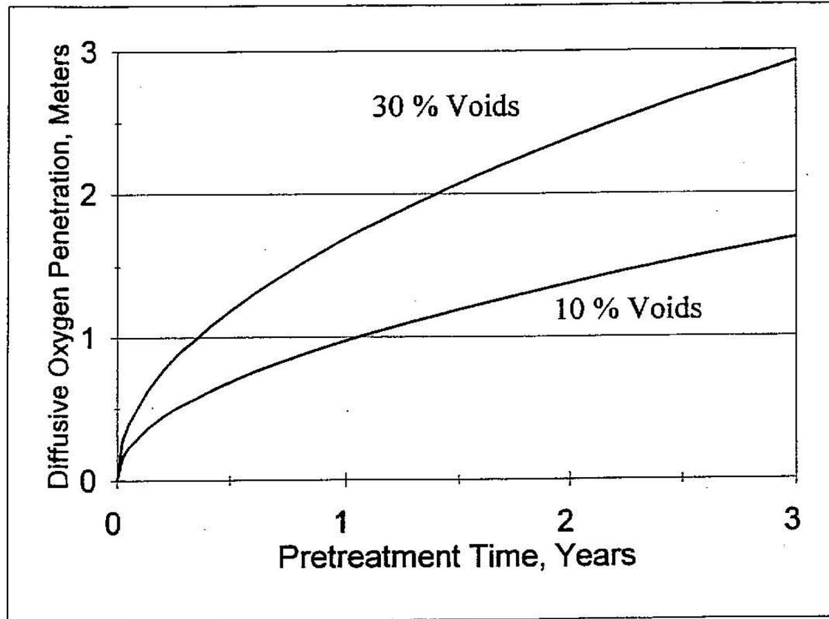
**Figure 8.2.** Diffusive oxygen penetration into an ore heap as a function of air-filled void space,  $v_g$ , and biooxidation pretreatment time, Pyrite = 1.0 wt pct (Bartlett and Prisbrey, 1995).
