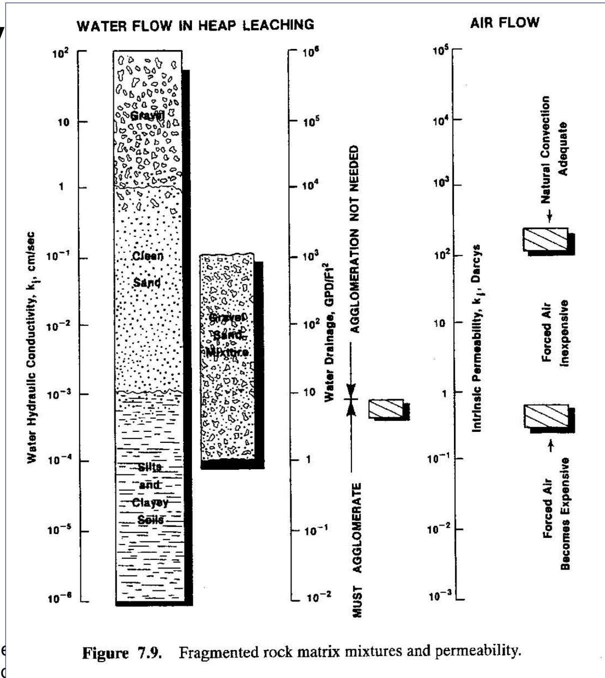
Figure 7.9. Fragmented rock matrix mixtures and permeability.
