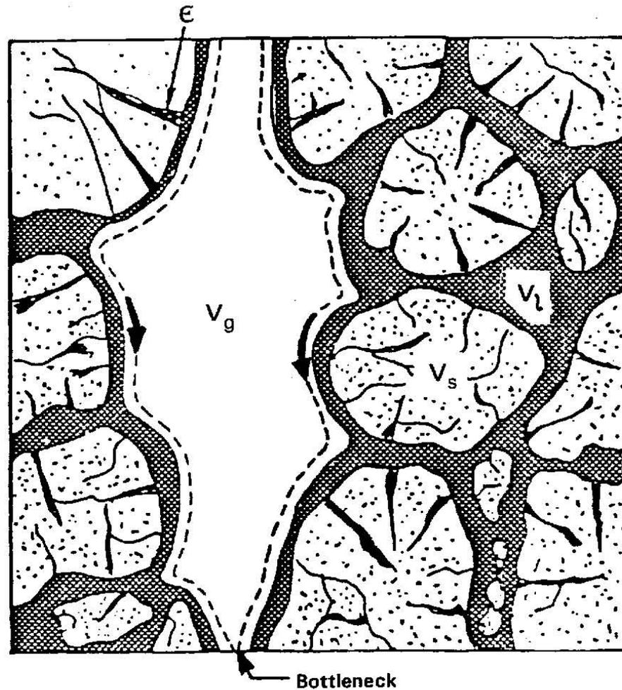
**Figure 7.1.** Schematic section of a heap showing space occupied by solids ( $v_s$ ), rock microporosity ( $\epsilon$ ), solution void space ( $v_l$ ) and air void space ( $v_g$ ) (Schlitt, 1984).
