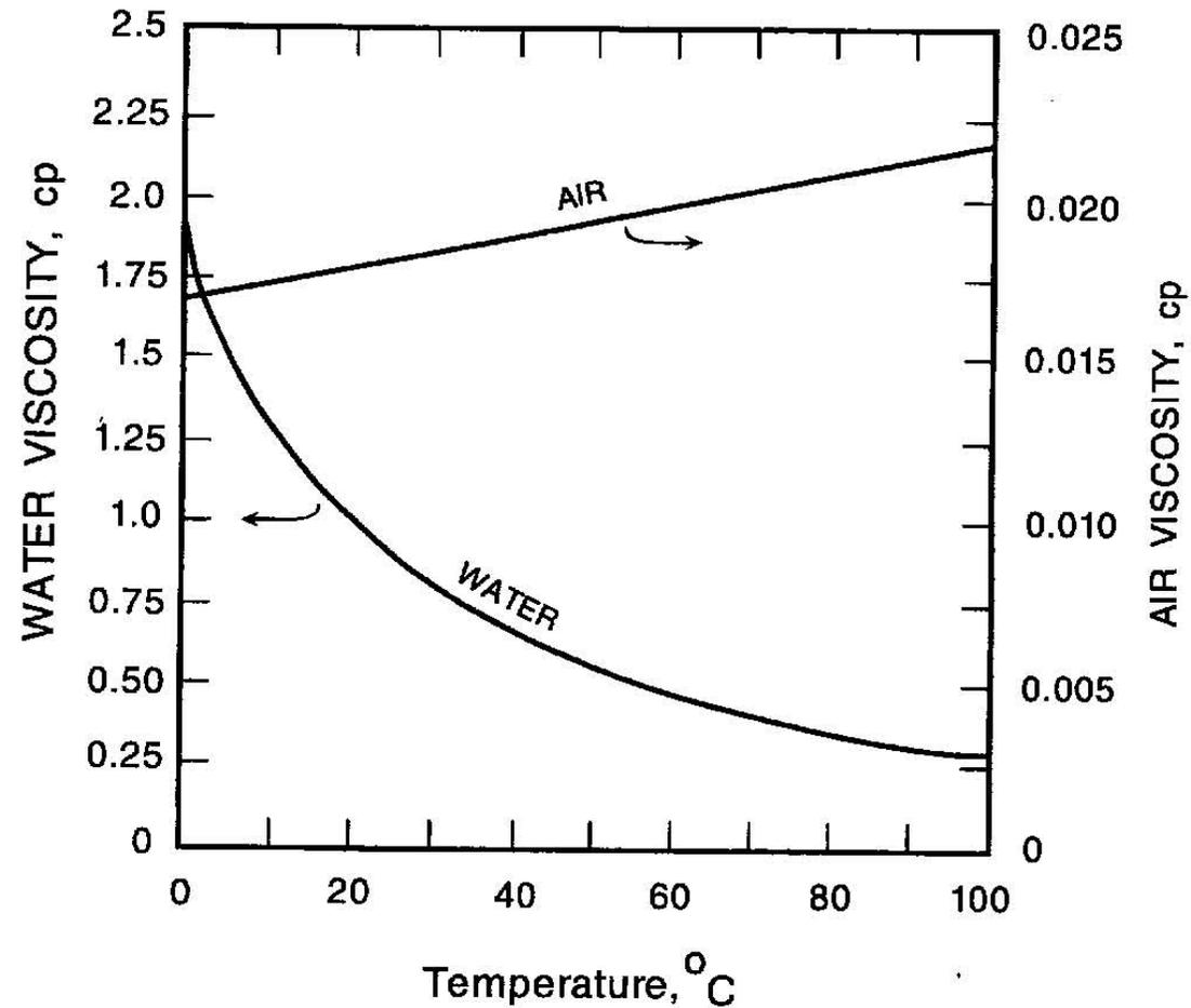
**Figure 7.4.** Temperature dependence of dynamic viscosities of water and air at 1 atm pressure (Bird et al., 1960).
