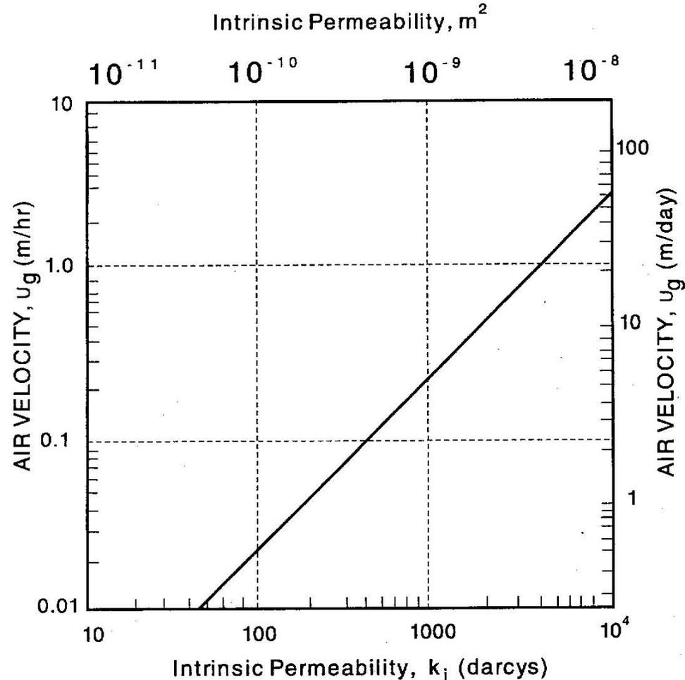
**Figure 8.4.** Natural advection limiting vertical air velocities and intrinsic permeability for:  $T_H - T_0 = 20^\circ\text{C}$  and 3% residual  $\text{O}_2$  in the exhausted air.
