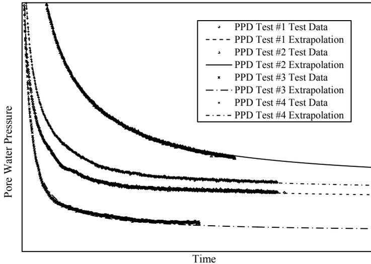
Figure 1. Extrapolations of Incomplete PPD Tests Shown With Experimental Test Data
