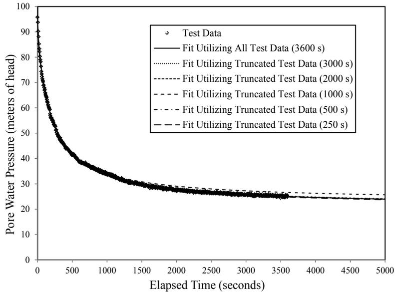
Figure 2. Extrapolations of PPD Test A Developed Utilizing Various Truncations of Experimental Data
