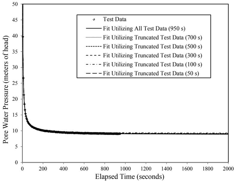
Figure 3. Extrapolations of PPD Test B Developed Utilizing Various Truncations of Experimental Data
