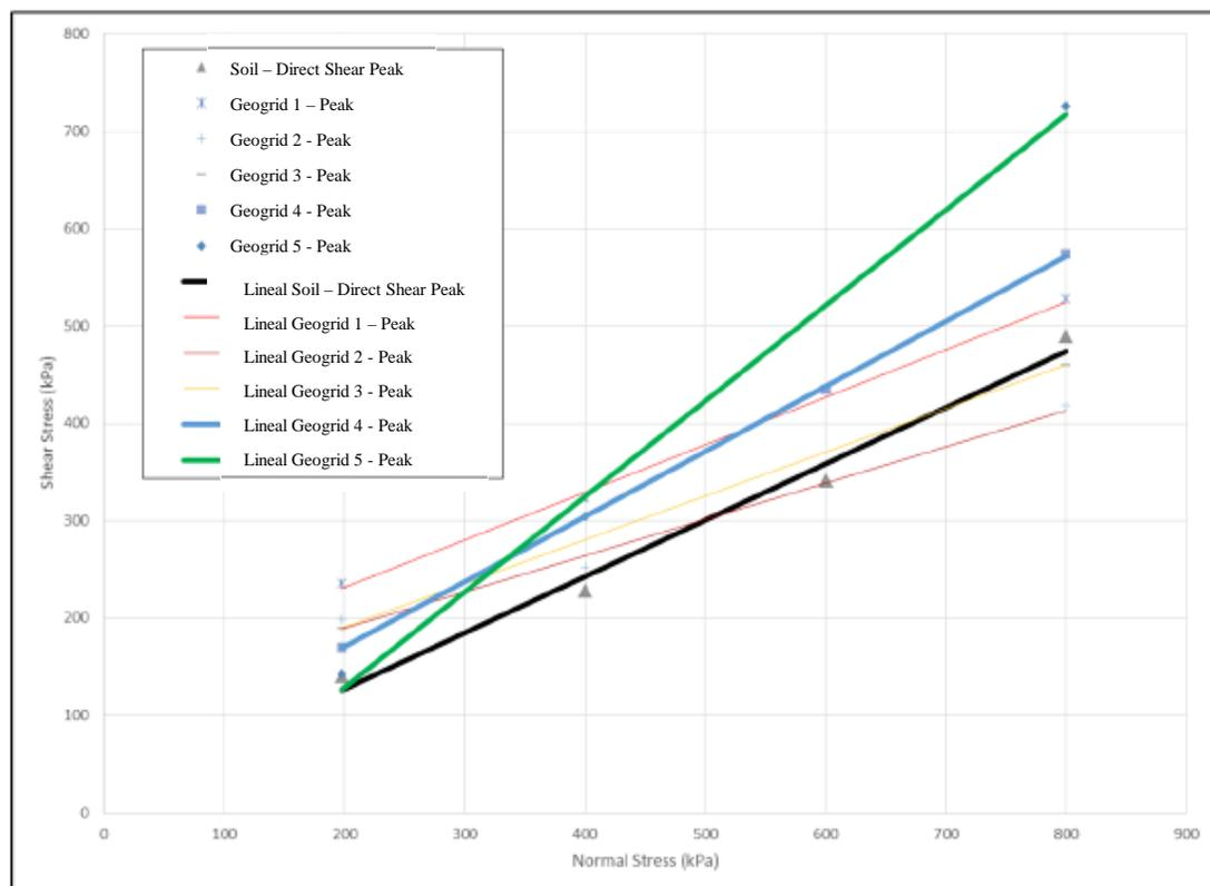
Figure 6. Summary of peak interface shear strength envelopes.
