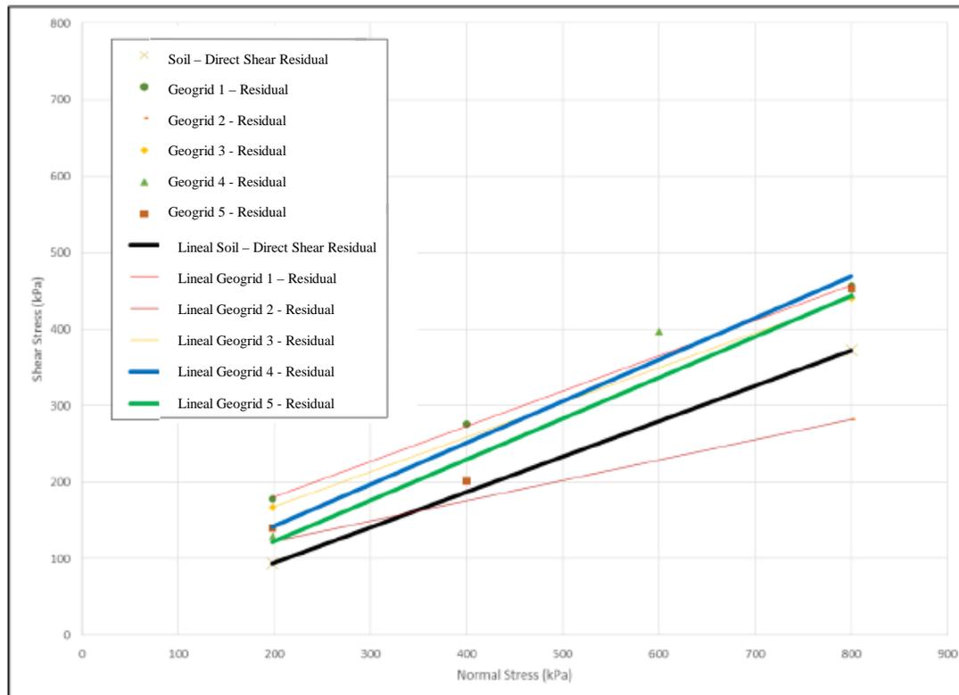
Figure 7. Summary of residual interface shear strength envelopes.
