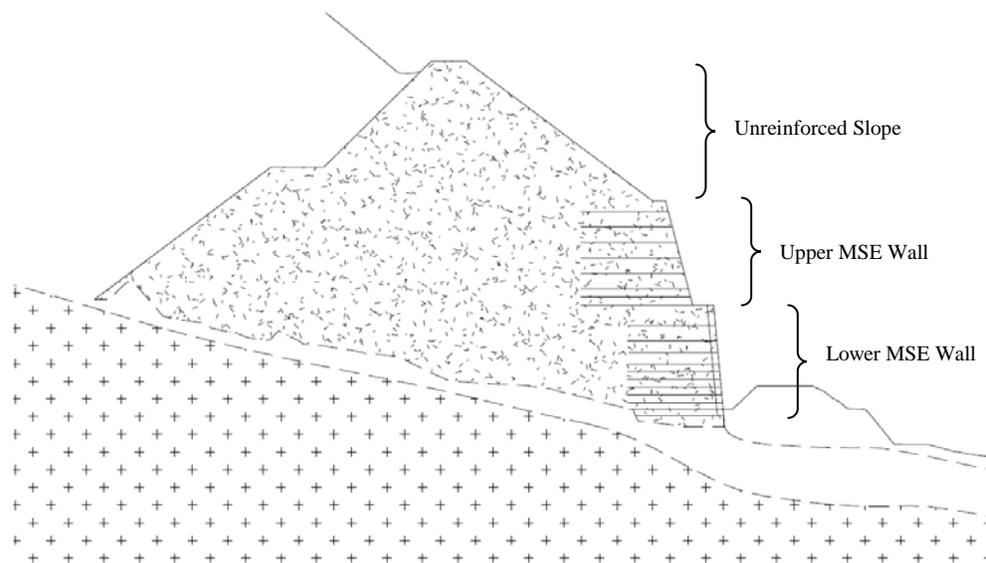
Figure 2. Cross section of the existing geogrid-reinforced toe buttress.
