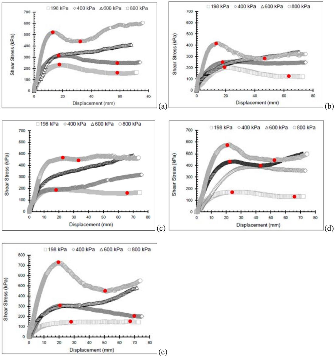
Figures 5 (a) to (e): Interface shear stress vs. displacement response using Geogrid 1 to Geogrid 5, respectively.
