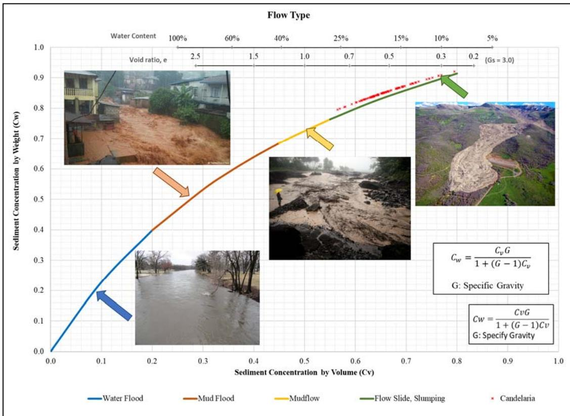
Figure 8. Flow type as a function of solids concentration (modified from Martin et al., 2019).
