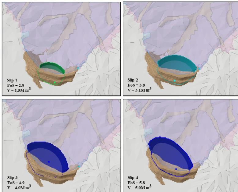
Figure 12. South Embankment – 3D LEA slip surfaces.
