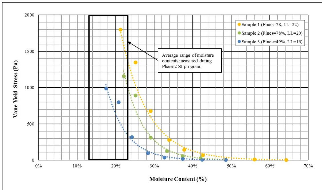
Figure 7. Vane testing results.
