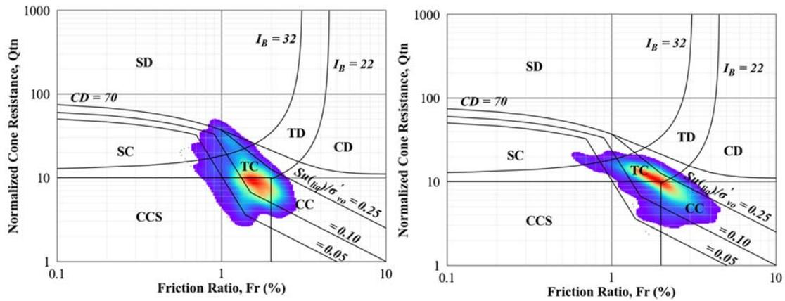
Figure 4. SBTn plots (Robertson, 2021) before (left) and after (right) Test Pad 1 construction.
