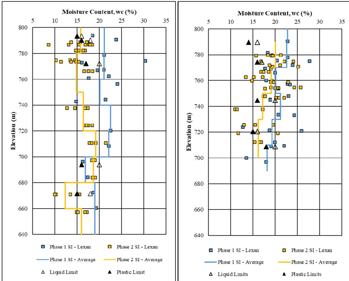
Figure 3. Moisture content results at Test Pad 1 (left) and Test Pad 2 (right).
