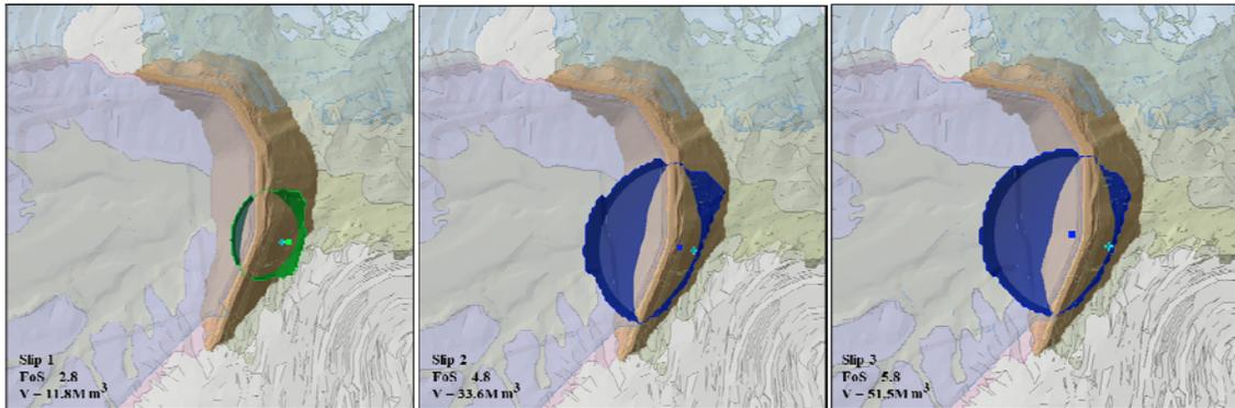
Figure 11. Main Embankment – 3D LEA Slip Surfaces
