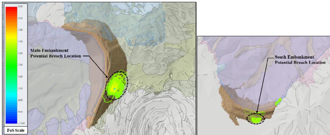
Figure 10. Potential breach location – Main Embankment (left) and South Embankment (right).
