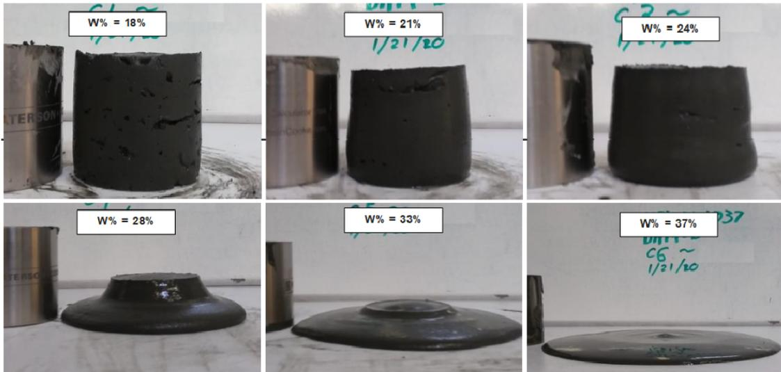
Figure 6. Boger slump test results with varying moisture content.
