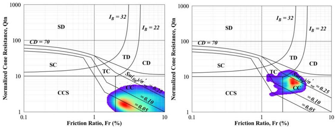
Figure 5. SBTn plots (Robertson, 2021) before (left) and after (right) Test Pad 2 construction.
