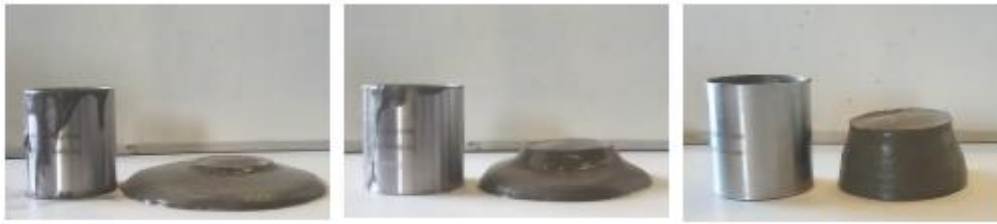
Figure 3 – Benchtop simulation of behaviour of tailings with variation in moisture content (MC) (images after Adams et al, 2018)
