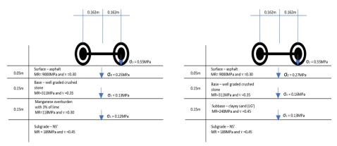
Fig. 5. Pavement cross-section with a lateritic clayey sand subbase (used in Brazil) and with a subbase composed of manganese overburden improved with 3% lime.
