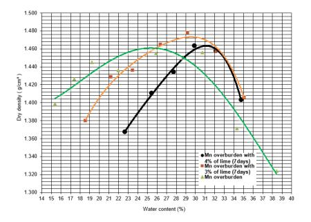
Fig. 2. Compaction curves - manganese overburden and manganese overburden-lime mixtures.
