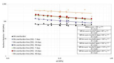
**Fig. 3.** Resilient modulus as a function of the deviator stress ( $\sigma_d$ ).
