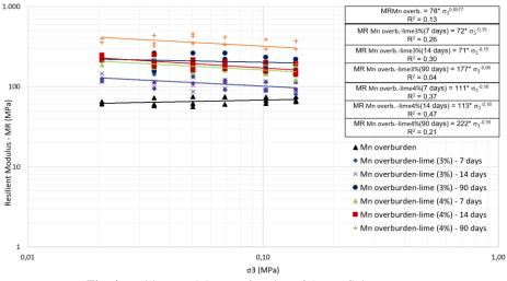
Fig. 4. Resilient modulus as a function of the confining stress ( $\sigma_{3}$ ).
