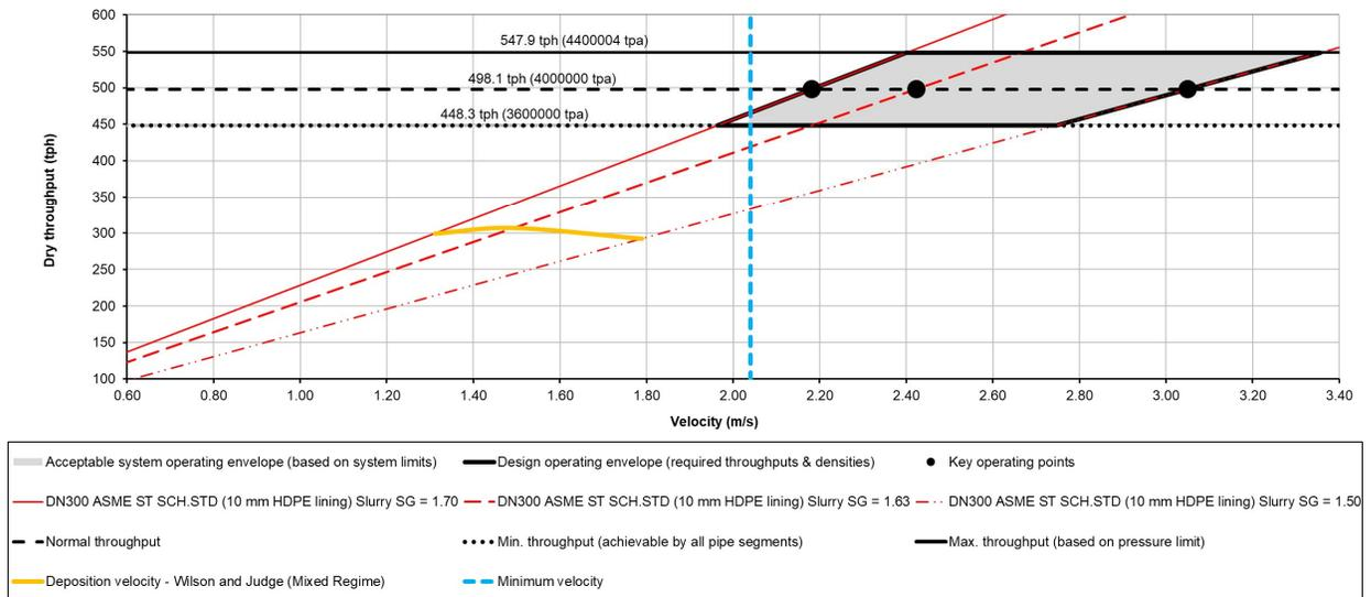
**Figure 16-1: Slurry operating envelopes for the DN300 STD SCHEDULE STEEL EPOXY COATED PIPE (WITH 10 MM HDPE LINING)**
