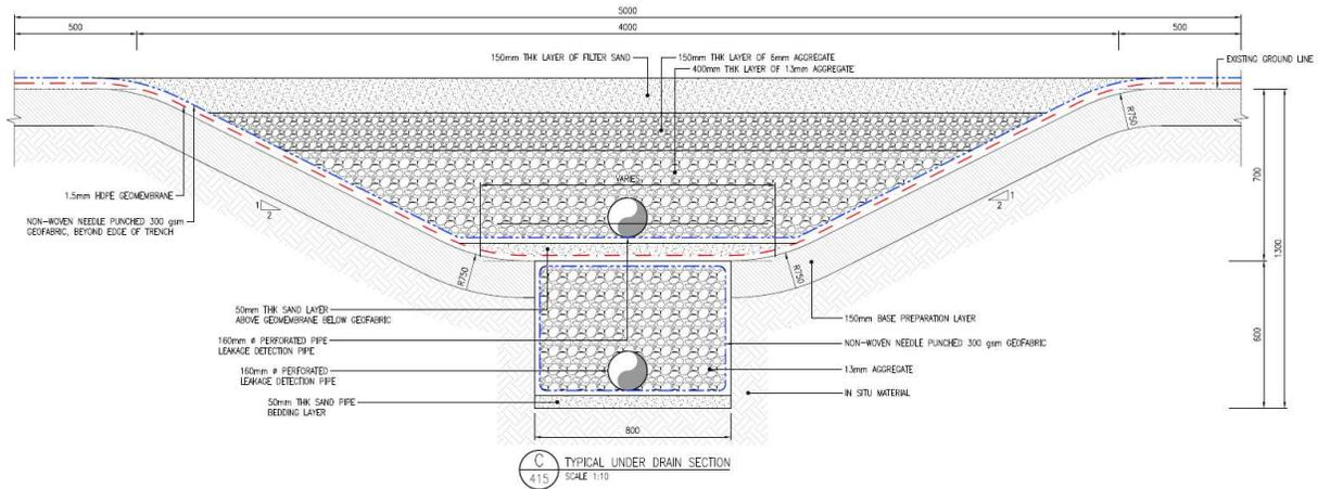
**Figure 10-1: Typical Underdrain Details**
