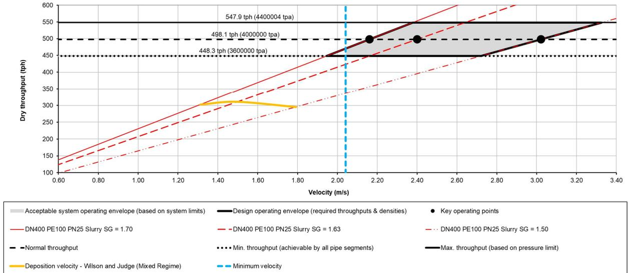
**Figure 16-2: Slurry operating envelopes for the DN400 PE100 PN25**
