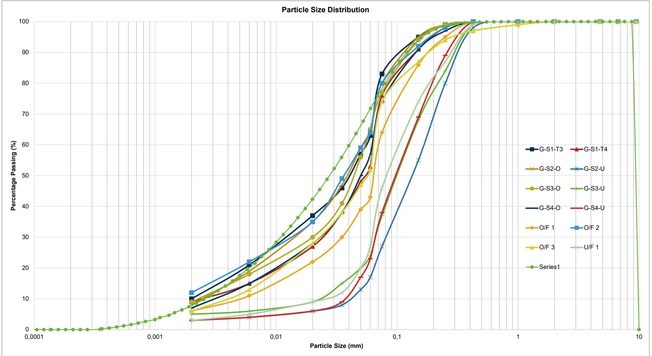
Figure 5-2: Tailings Particle Size Distribution
