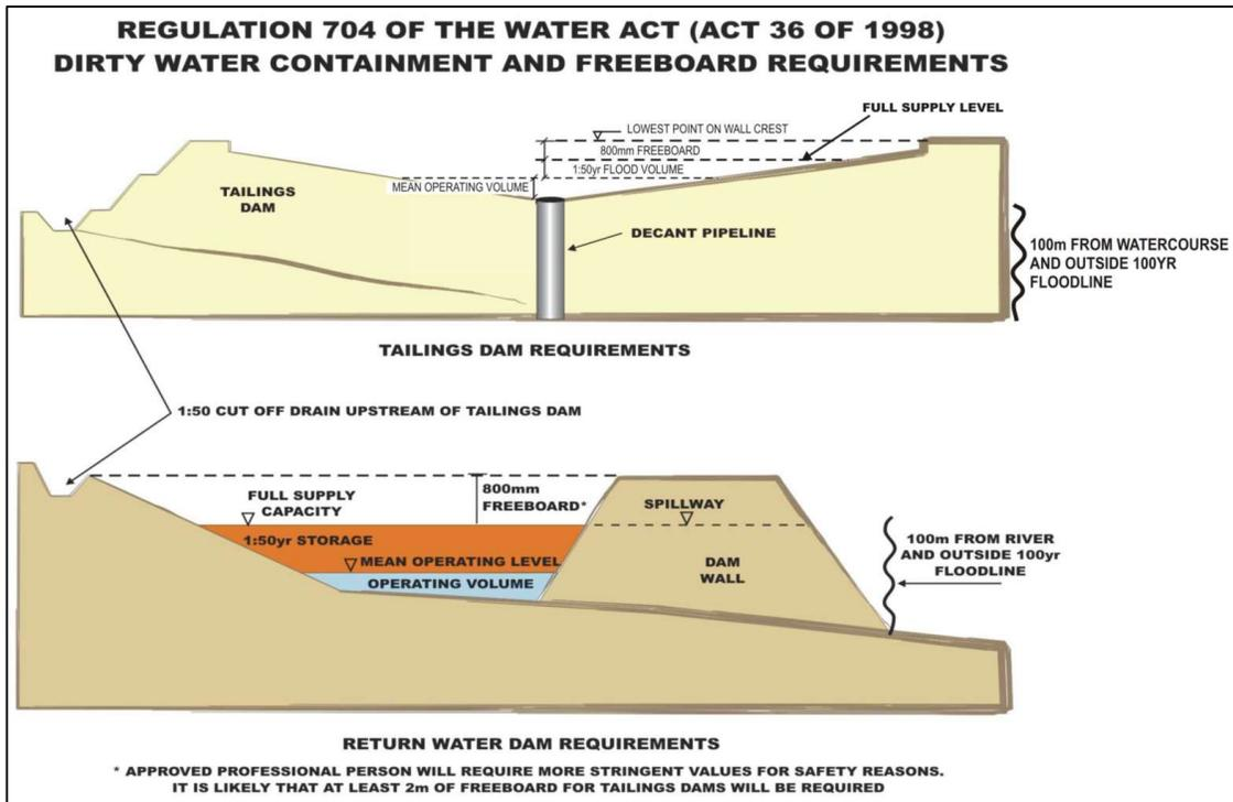
Figure 13-1 Dirty Water Containment and Freeboard Requirements as per GN704
