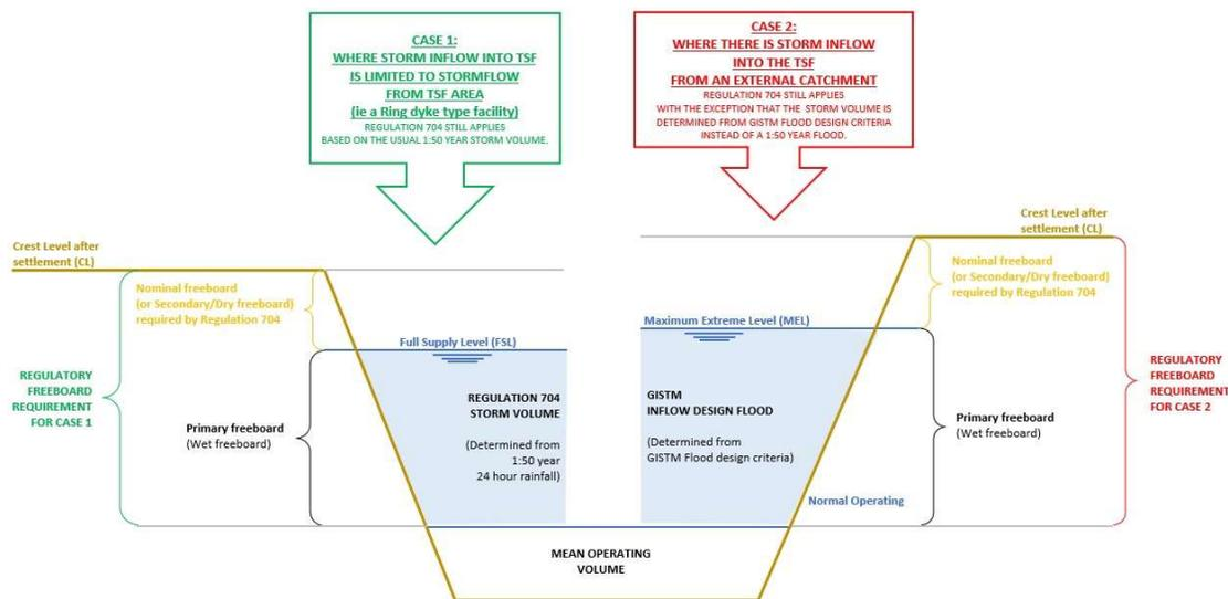
Figure 13-2 Dirty Water Containment and Freeboard Requirements as per GISTM
