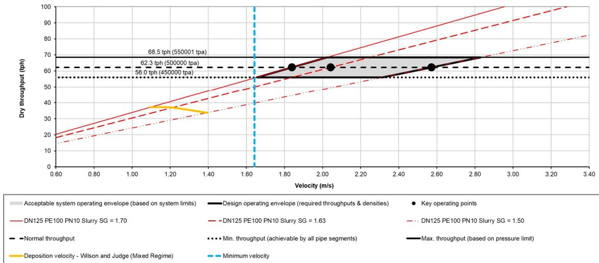
**Figure 16-5: Slurry operating envelopes for the DN125 PE100 PN10 (with 8 number of Offtake pipes to cyclones)**
