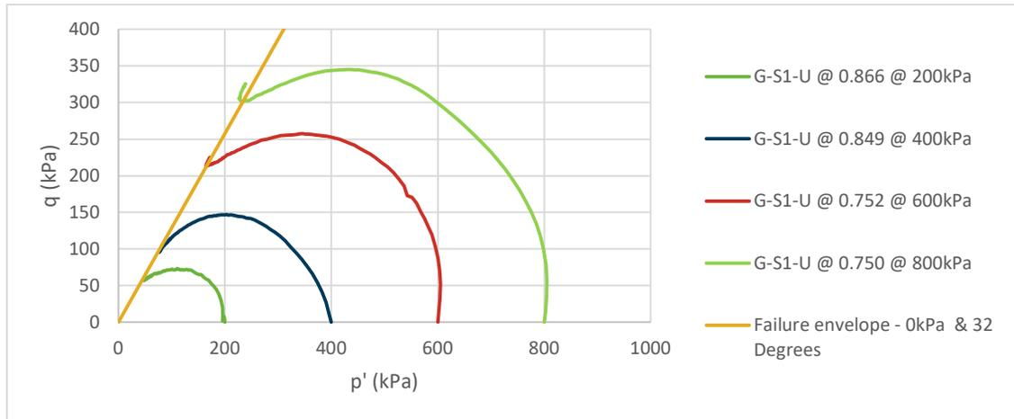
Figure 5-4: CU Triaxial Tests – Underflow
