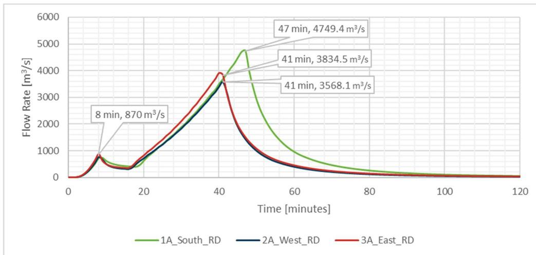
Figure 14-2: Breach outflow hydrographs for Rainy-Day failure scenarios
