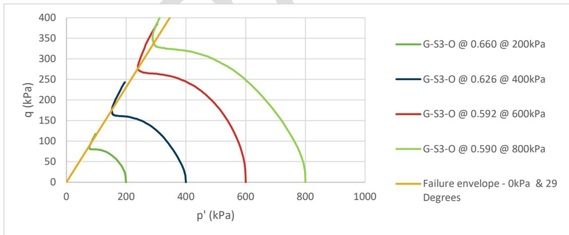
Figure 5-5: CU Triaxial Tests – Overflow
