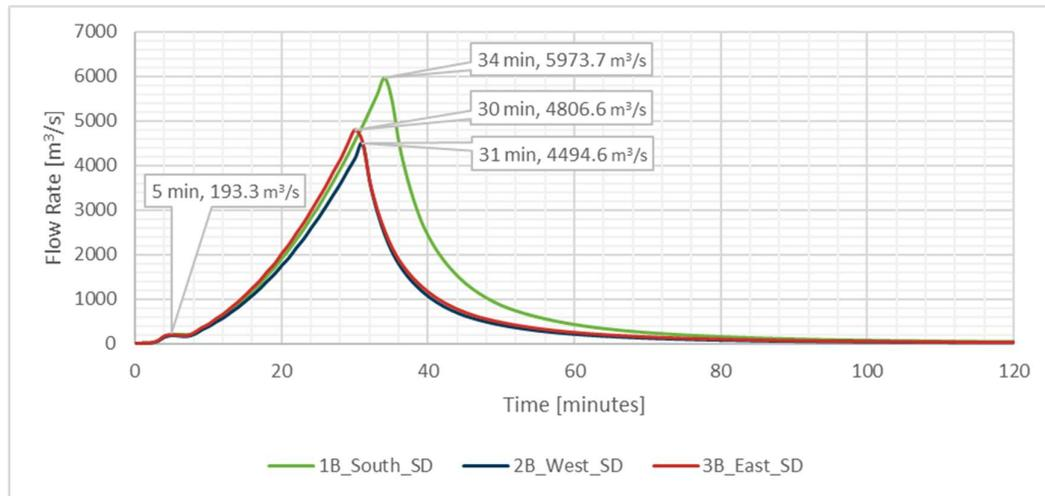
Figure 14-3: Breach outflow hydrographs for Sunny-Day failure scenarios
