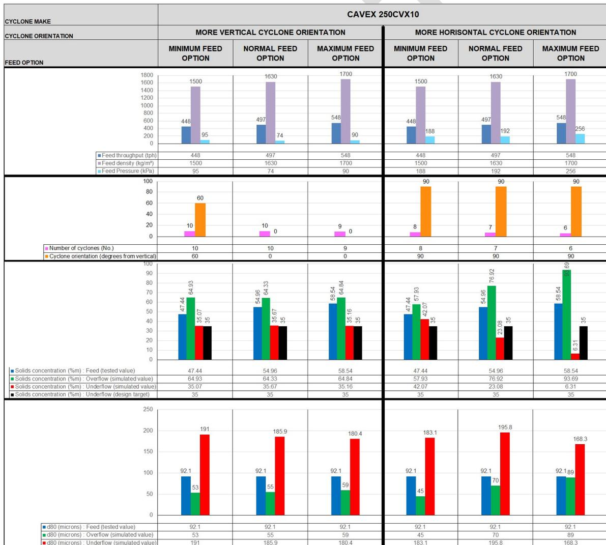
Figure 16.6: Graphical summary of cyclone simulation results (from Weir minerals)
