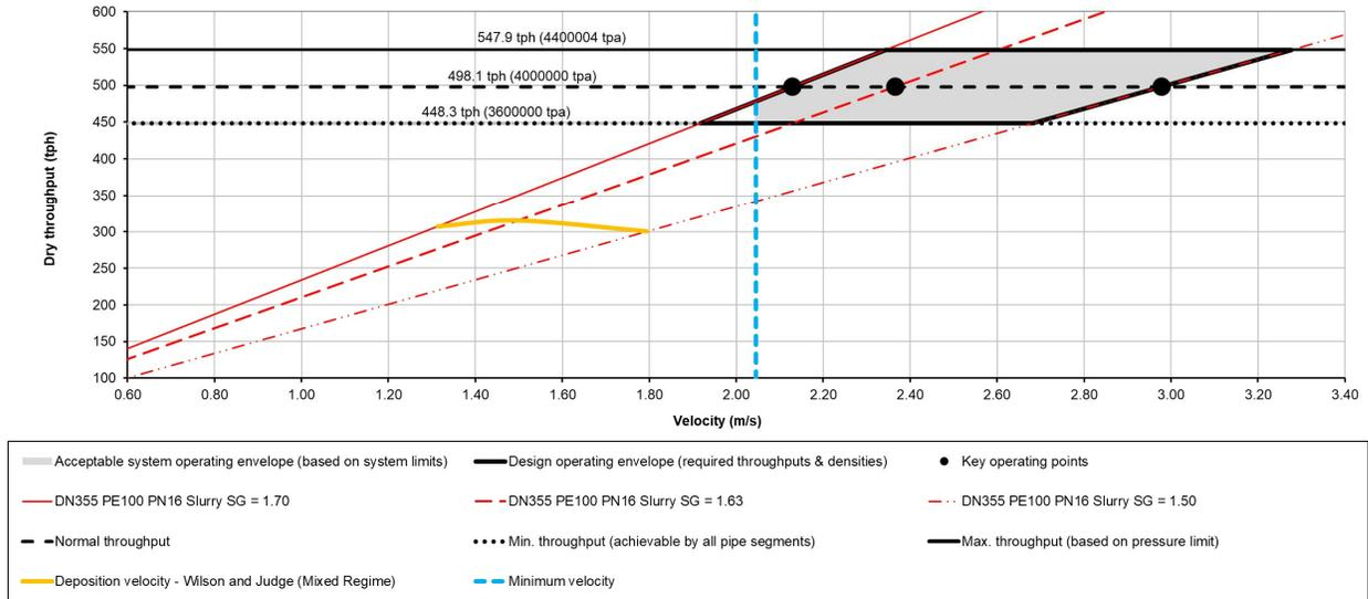
**Figure 16-3: Slurry operating envelopes for the DN355 PE100 PN16**
