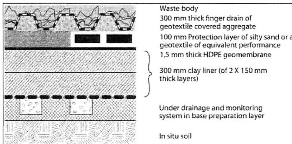
Figure 7-1: Standard Class C Barrier System
