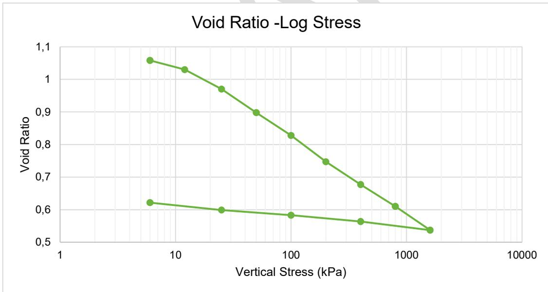
**Figure 5-9: Void Ratio v Log Stress - Underflow**
