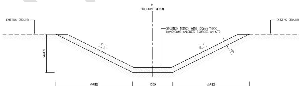
**Figure 12-4 Typical cross-section of stormwater drains around TSF 2**
