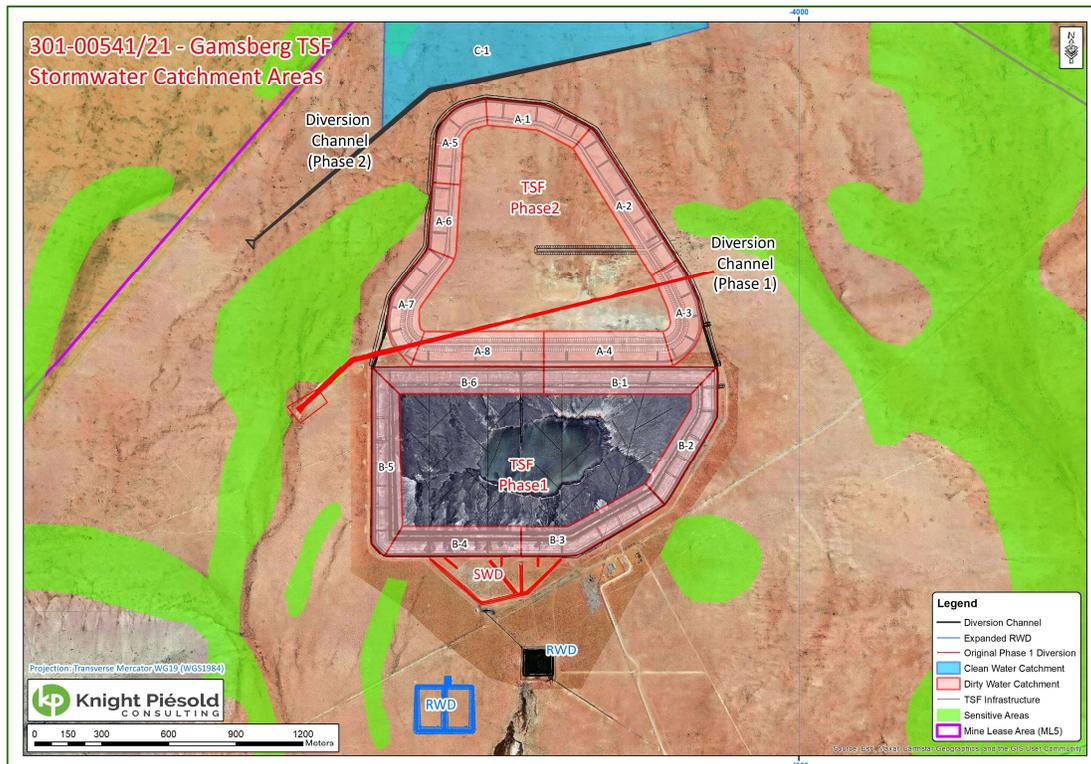
**Figure 12-3 Contributing catchments and channel arrangement for both phases**
