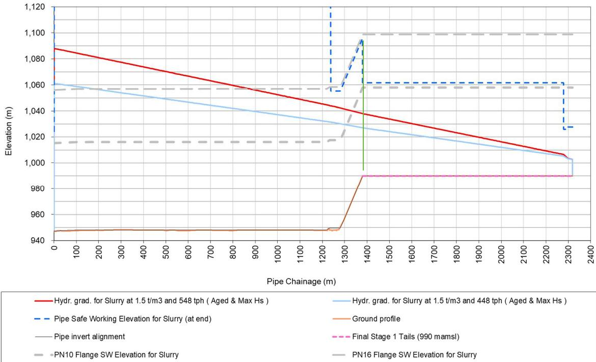
**Table 16.2: Hydraulic gradient– Proposed Tailings slurry ringfeed system (from chainage 0 on KP long section drawing to the furthest deposition point on the TSF along the Western branch)**
