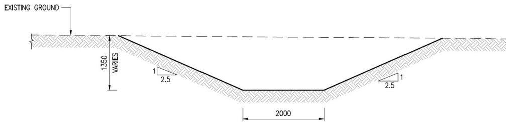
**Figure 12-7 Typical cross section of clean water diversion channel**
