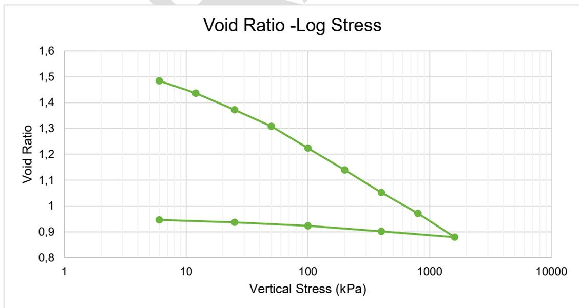
**Figure 5-7: Void Ratio v Log Stress - Underflow**
