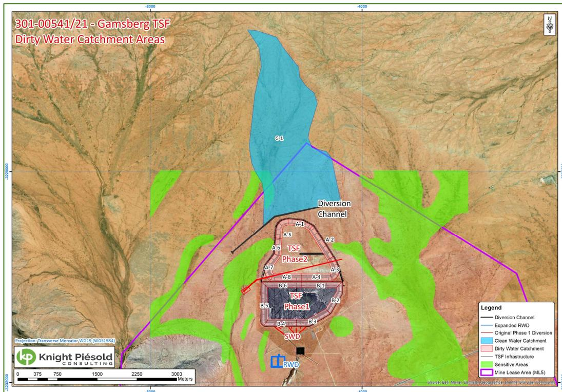
Figure 12-6 Location and catchments of new clean diversion channel
