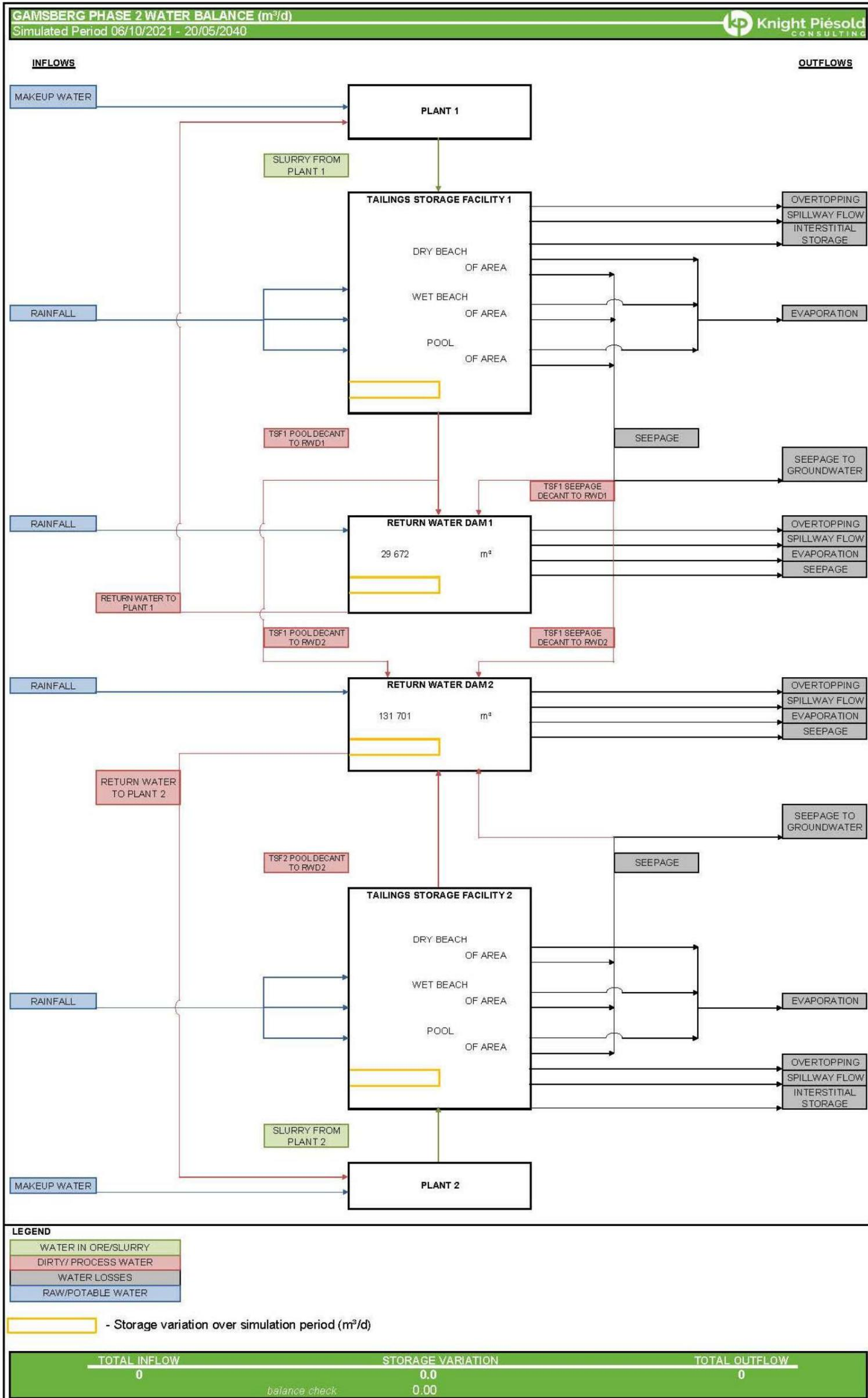
Figure 13-3 Gamsberg Phase 2 Water Balance Schematic
