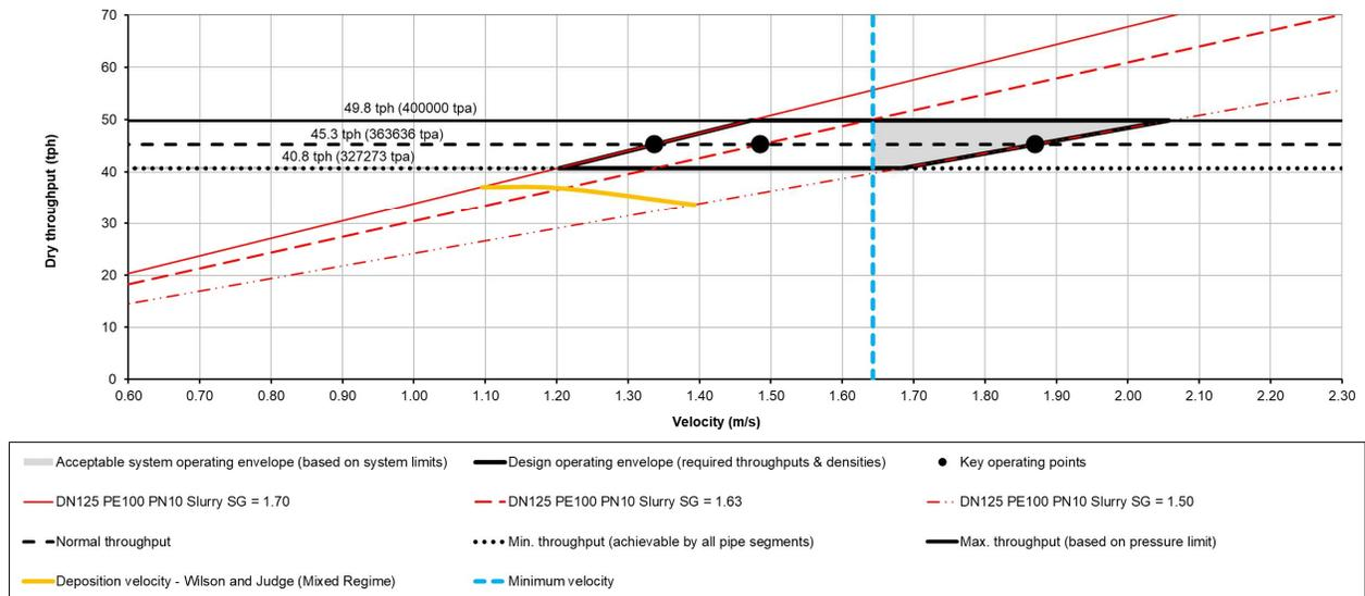
**Figure 16-4: Slurry operating envelopes for the DN125 PE100 PN10 (with 11 number of offtake pipes to cyclones)**
