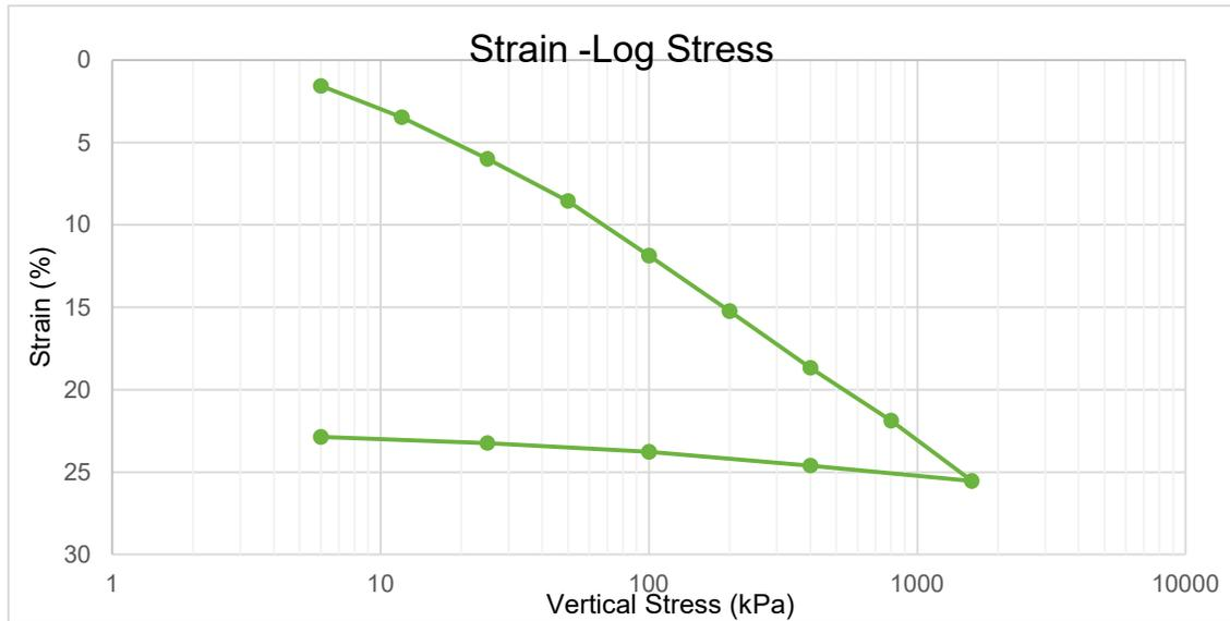
**Figure 5-6: Strain v Log Stress - Underflow**
