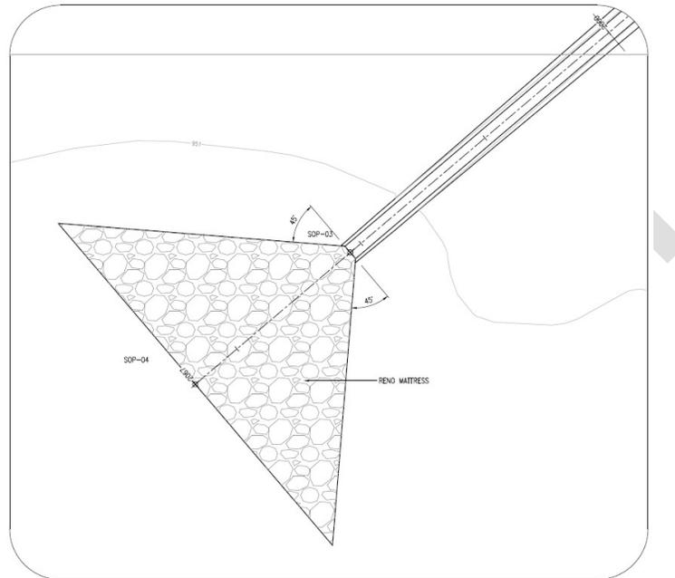
**Figure 12-8 Outlet of clean water diversion channel**
