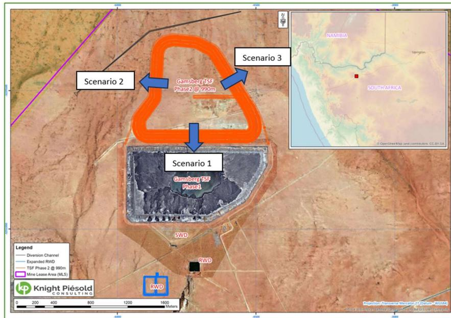
Figure 14-1: Schematic indicating recommended breach positions.
